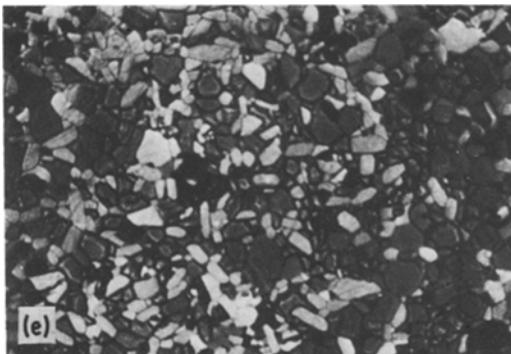
Figure 7 Microstructures of the oxidized samples of different compositions shown in Fig. 5 b to f (a)  $x = 0.5$  (b)  $x = 1.0$  (c)  $x = 1.5$  (d)  $x = 2.0$  and (e)  $x = 2.5$ .
